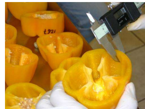
Digital caliper AutoTec 150 mm (d=0.01 mm)
